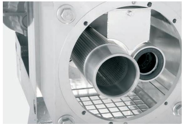
Granulating cylinder (left) and pressure cylinder (right)
